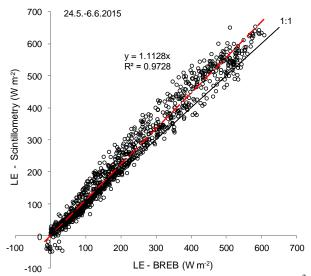
Fig 4 The regression between latent heat (LE) flux (W.m<sup>-2</sup>) derived by the BREB method and the scintillometry
