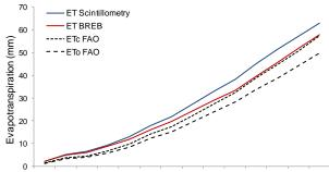
24.5. 25.5. 26.5. 27.5. 28.5. 29.5. 30.5. 31.5. 1.6. 2.6. 3.6. 4.6. 5.6. 6.6. Fig 2 The cumulative evapotranspiration (mm) derived by the scintillometry – solid blue line, the BREB method – solid red line, reference ETo and ETc by FAO56 – black dashed lines, for winter wheat
