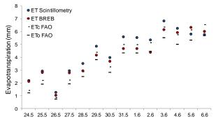
Fig 1 The daily totals of actual evapotranspiration (mm) derived by the BREB method, the scintillometry, and reference ETo and ETc by FAO56 for Polkovice site in 2015
