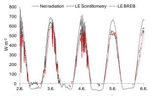
Fig 3 The comparison between LE (W.m<sup>-2</sup>) derived by the BREB method and the scintillometry from 2.6.2015 12:00 to 6.6.2015 12:00 in Polkovice
