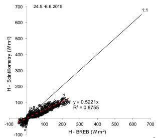
Fig 5 The comparison between sensible heat (H) flux  $(W.m^{-2})$  derived by the BREB method and the scintillometry
